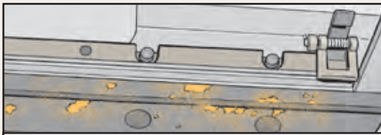
Wipe away any dirt or grease that will keep SFL from sticking
