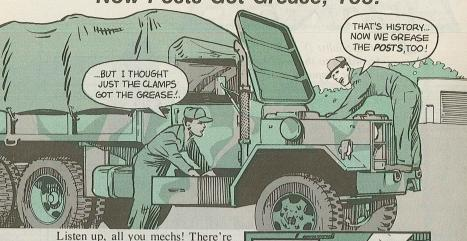
a couple of new words on using GAA to prevent corrosion on battery hookups:
