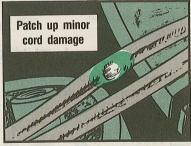
If a wire's exposed or insulation's frayed-but there's no evidence of wire damage-go ahead and tape. Use at least 2 layers, and spread the tape an inch beyond the damaged area in both directions. Skip the taping if you see dry rot, damaged wire or 2 or more bare wires.
