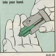
Set the plug on a flat surface. Squeeze the locking pins back into the plug. The detent ball will drop to the bottom of the plug.
