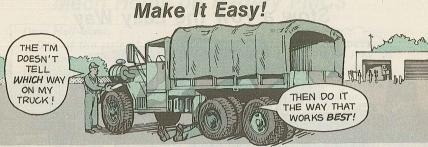
Can't decide which is the right way to install prop shaft coupling bolts and nuts on your vehicle? If your TM doesn't specify a certain way, it makes no difference whether the nut is toward the front or the rear.
