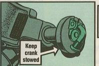
If you leave the crank open, it snags on just about anything...and bends or breaks. No crank, no traversing, no mortar.
