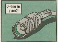
Smooth the way even more with a light coat of silicone on the rubber. Don't get any on the contacts, tho. If you do, wipe it off ASAP.
