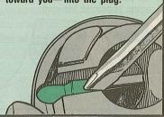
(2) Install the retaining ring. Be sure it's seated against the tumbler shield and the cylinder shield. If it's not seated good, you can't seat the cylinder.
