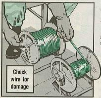
Look the wire over closely as you put it back on reels. Look for cuts, splices, worn spots or insulation damage.
