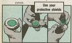
if yours is damaged or lost, try a substitute. The cellophane from a cigarette pack can be cut to size and glued over a damaged shield.
