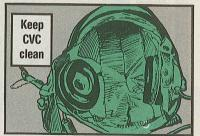
Are ear pads torn or missing? Is the boom assembly dirty, broken or corroded? How about ball joints? Look inside earphones for dirt and moisture.
