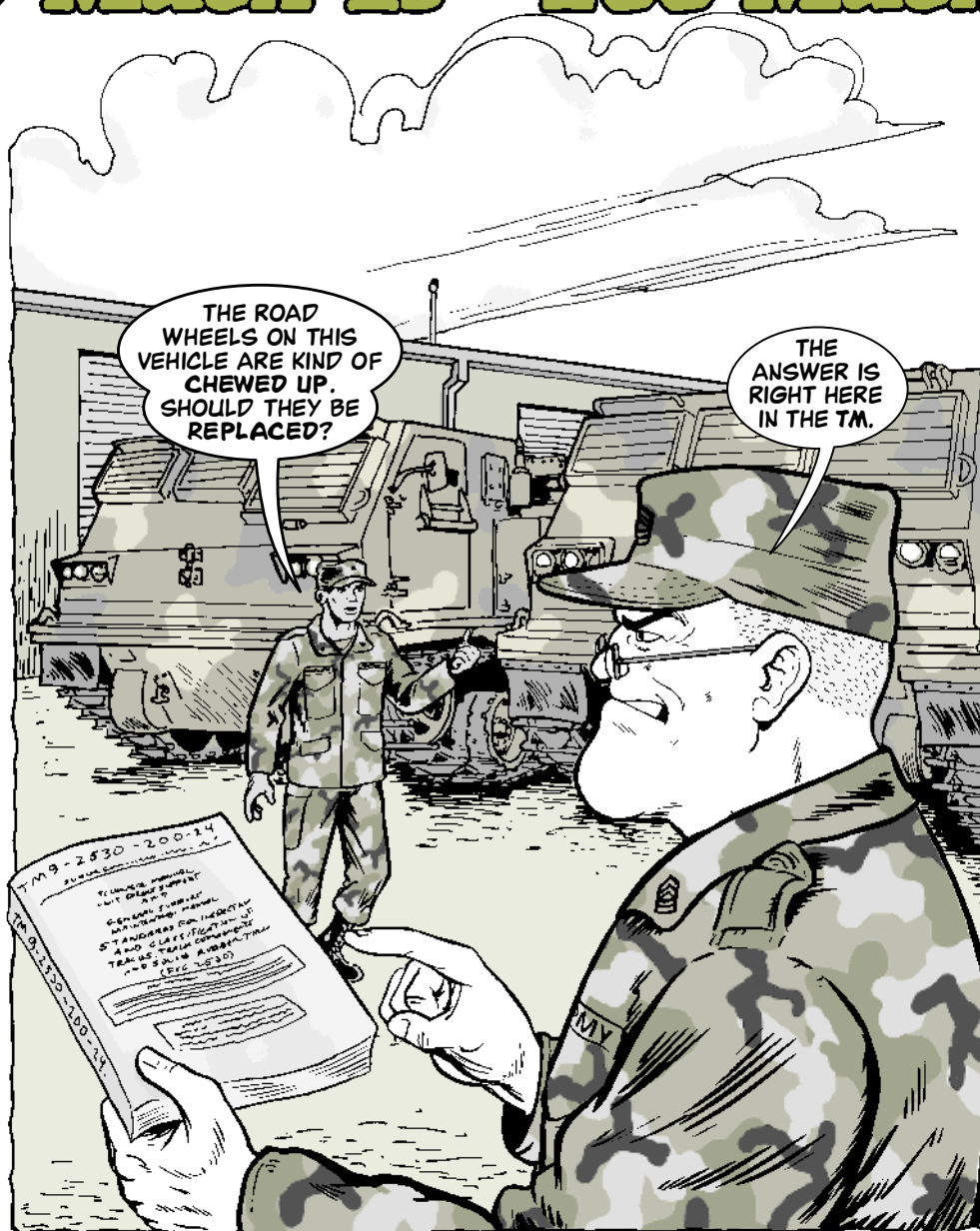
Check for separation that extends 75 percent around roadwheel
