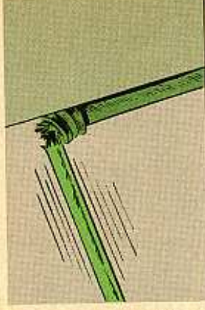
Also puts a strain on the bracket and could lead to a worn, frayed, and maybe broken cable.
