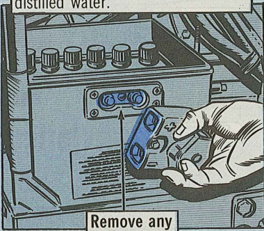
Remove any corrosion
