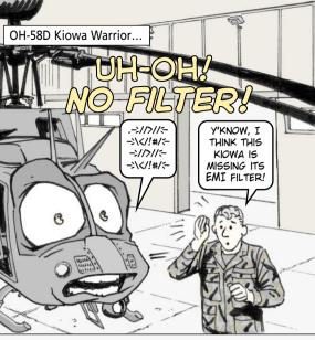
Some Kiowas' Block 1 Air-to-Air Stinger (ATAS) interface electronics assemblies (IEA) were installed before it was decided to add an electromagnetic interference (EMI) filter to the J1 connector.
