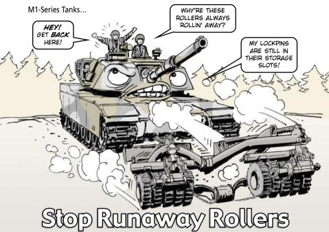
There are a whole lot of steps to follow when installing the mine clearing roller on your M1-series tank. One of the most important is securing the angle brackets with two lockpins, NSN 5315-00-628-4001.
