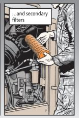
REPLACE THE PRIMARY AIR FILTER ELEMENT, NGN 2940-01-580-0028, ONCE A YEAR OR AFTER SIX CLEANINGS, WHICHEVER COMES FIRST. SAME GOES FOR THE SECONDARY FILTER, NGN 2940-01-579-8964.
