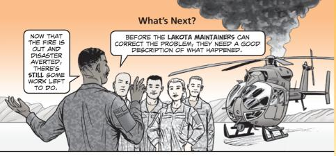
YOU NEEP TO INCLUDE **ALL** THE STEPS TAKEN AS WELL AS THE MAXIMUM TOT REACHEP AND ITS PURATION. ALL OF THIS INFORMATION IS NEEDED TO **DETERMINE** THE PROPER INSPECTIONS AND MAINTENANCE ACTIONS NEEDED TO RETURN THE AIRCRAFT TO SERVICE.
