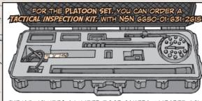
THE KIT INCLUDES AN UNDER-DOOR CAMERA, INFRARED POLE CAMERA, FIBERSCOPE AND A REVERSE PEEPHOLE SCOPE.
