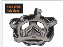
Don't fold the mask when you put it in the carrier. That ruins the mask. The mask goes in the carrier in the upright position with the eye lenses facing away from your body when worn in the shoulder, leg or loadbearing harness positions.
