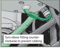
We put a stop to this rubbing problem by turning the oil return line's elbow fitting, NSN 4730-00-231-4009, counterclockwise slightly. That raises the oil return line enough to keep the two lines from touching.
