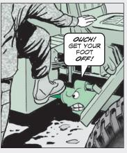
To save costly repairs and downtime, get on the forklift from the roadside and keep your feet off the cylinder rods.
