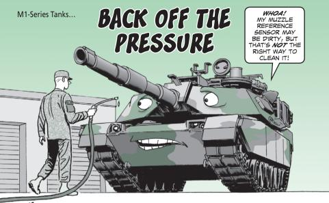
High-pressure water is a sure way to remove stubborn dirt from your tank, crewmen. It's also a sure way to damage components like the muzzle reference sensor (MRS). The PMCS section of the -10-1 TMs specifically prohibits the use of high-pressure
