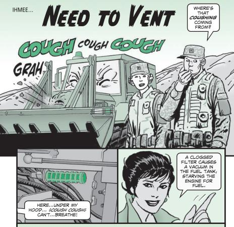
**O**perators, the excavator's fuel tank needs to vent...but that's OK!
