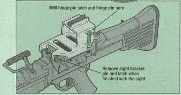
Make sure your unit knows there is a place on the mounting bracket to store the M60 pin and latch while using the sight. And make sure they remove the bracket pins and replace them with the M60 pin and latch when they're through with the sight. Check that all pins are present when the sight's turned in.
