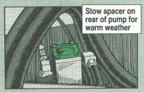
transfer case to its stowed position behind the pump. This engages the pump and lets the oil cool the gears.
