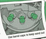
We've sealed out sand with barrel caps for the M16 rifle. Any time we're in a dusty, sandy area, we put caps on the three smoke discharge hole spouts. The caps fit tight after a 1/2-in long slit is made on four points of the cap. When it's time to smoke, it's no problem pulling off the caps.
