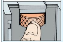
Barrel locking spring—If the spring can't hold the barrel in place, the barrel can turn during firing and headspace is lost. So test the spring by getting the correct headspace and then trying to unscrew the barrel. If the barrel turns, the spring is weak or loose.
