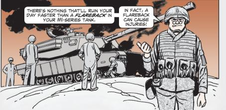
Flareback happens when the fuel-rich gases formed by firing the main gun enter the crew compartment, mix with oxygen, and then are ignited by some source.
