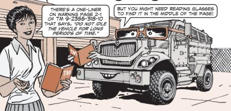
YOU'RE ASKING FOR TROUBLE WHEN YOU RUN THE MRAP'S DIESEL ENGINE FOR LONG STRETCHES AT LOW IDLE.
