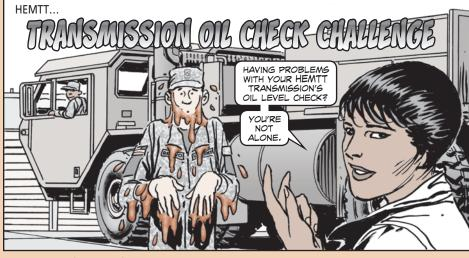
Word from the field is that HEMTT users have found transmission oil blows out of the vent at startup. That's a sign that the oil level could be too high.
