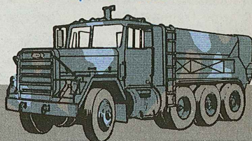
M919, 8x6, mobile concrete mixer
