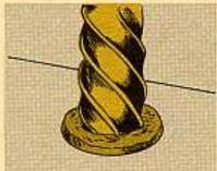
Minor surgery is needed if the fitting snaps below the nut. Poke the remover into the hole and start turning counterclockwise.
