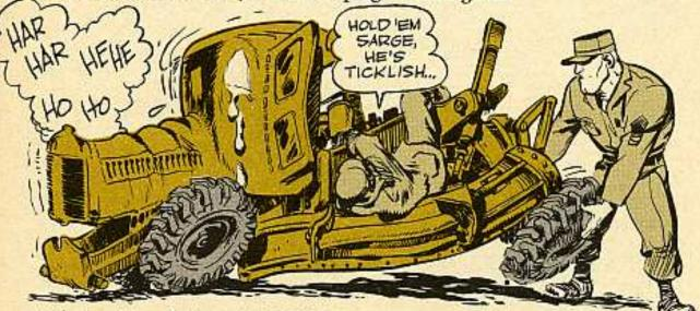
Substituting a drain cock, FSN 4820-033-5972 (ENG), and a bushing, FSN 4730-193-0871 (ENG), for the plug makes the draining routine as easy as tapping a keg of brew. And, the toughest part of making the substitution is getting at the drain plug. Putting the drain cock on is a breeze.
