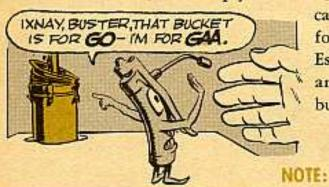
cans and guns. Use the same container for the same lube right down the line. Especially so in the case of GAA, Am 2 and Am 3. It should have the same bucket and gun (lubricator) every time.
