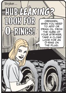
If that O-ring is missing or damaged, you won't get a good seal and the hub can leak. If the hub goes dry, it'll burn up.
