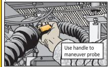
Before you hit the road, make sure the probe is locked up for travel. Otherwise, it can bang around, which ruins its membrane. After you fasten the probe's seatbelt, give it a tug to make sure it's locked in. Sometimes the seatbelt looks like it's secured when it's not.
