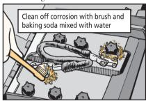
While you're checking the batteries, don't forget the ground straps. If they're broken, frayed, loose or corroded, the batteries will be weakened. Do not use the straps to maneuver batteries. You'll just break them.
