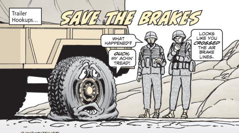
is the word to keep in mind when you hook up the brake air hoses from a trailer to your  $2^{1/2}$ - or 5-ton truck. If you cross the air lines, the trailer brakes will lock up, burn out or ruin the tires.
