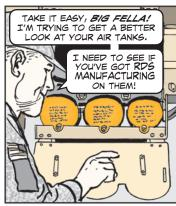
Caiman MRAP users need to take a close look at the vehicle's primary, secondary and wet tanks. These tanks are known to rupture, causing the air brake system to fail. Not good!
