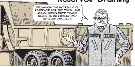
Since there's no drain plug, disconnect the oil line at the bottom of the tank. Make sure you let the oil cool before you loosen the line, so you won't get a hot oil bath. While reconnecting the line, be sure not to cross thread the fitting. If you strip the threads, the truck will have to go to support to get the hose replaced.
