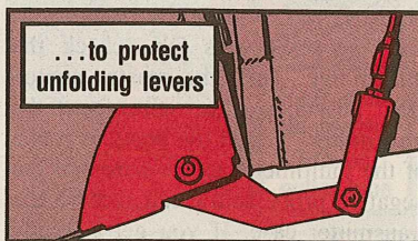
Put blocks under rear of bridge bay...
