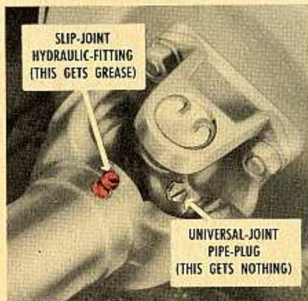
Fig. 1—The M38A1's universal joint has a not-to-be-removed plug, and no hydraulic fitting.
