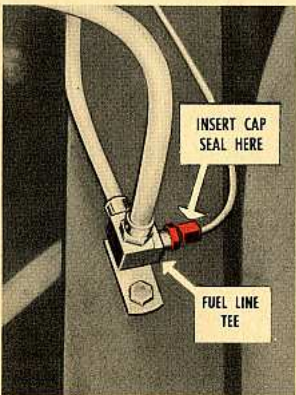
2 1/2-ton (GMC) —The cap seal is set in the primer-pump rear-line at the fuel-tank-line tee.
