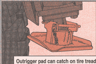
Outrigger pad can catch on tire tread
