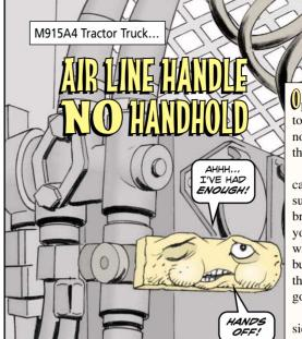
Uperators and mechanics, the tractor truck's air line cutoff handle is no handhold for climbing aboard the catwalk.
