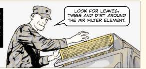
Before the day's run, remove the element and tap it with your hand to get rid of trapped dirt. Do not bang it against the cab! You'll bend its sealing edge or crush filtering material.
