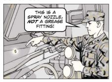
Grease either clogs the nozzle or ends up on the windshield when you push the washer fluid button to clean the windshield
