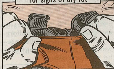
Stretch faceblank to search for signs of dry rot
