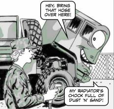
Clean mud off the vehicle as soon as possible. Pay special attention when cleaning to the wheels, brakes, axles, universal joints, steering mechanism, radiator and oil cooler.
