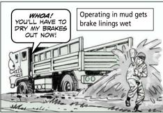
• Operating in mud gets the brake linings wet. That greatly reduces braking power. To dry the brakes, first find a dry area, or at least an area where the brake drums will be totally out of the mud. Drive the truck about 500 feet, applying the service brakes frequently. If you still have problems with the brakes, call in your unit mechanic.
