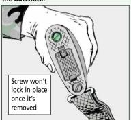
Once the screw is removed, it's no longer self-locking. It won't hold and the buttstock can turn while firing.
