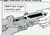
If the trigger assembly is put together wrong, the weapon fires automatic when it's not supposed to. That's dangerous.
