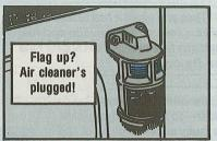
So eyeball that air cleaner indicator. If the colored flag is locked up in view, your air cleaner's plugged. Get it fixed—element cleaned, dried out or replaced.
