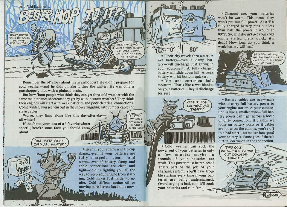
• A weak battery can freeze into a block of ice. A fully charged battery will take cold down to -90°F. This's because the electrolyte (battery acid) in a fully charged battery is about one-quarter sulfuric acid. As a battery discharges, the electrolyte becomes less acid and more water. Charging returns the electrolyte to the right balance of acid and water. This's part of the "chemical energy" that turns into electrical energy when you hit the starter switch.
