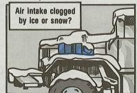
snow shutting off your engine's air supply? You can wind up with a plugged air cleaner even if you just got a spanking-clean element. Moist air sucked into your cleaner can freeze on the element. Snow can do the same thing. Either way, it's the same as a dirt-plugged element. Air can't get thru!
