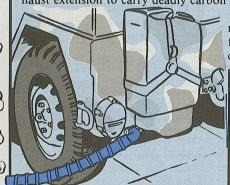
A snug fit over the tailpipe is a must—to prevent a leak. Here are flexible tubes to fit some common-size tailpipes:
