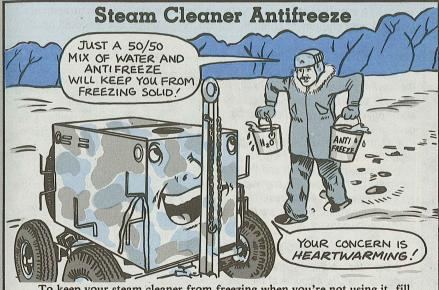
To keep your steam cleaner from freezing when you're not using it, fill it with a 50/50 mix of water and antifreeze. Pump the mix out and save it for later before you use the cleaner.
