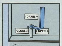
When it's cold outside, be sure to drain the water from your M12A1 decon apparatus. Water left standing in the M12A1 freezes only a few degrees below 32 °F or 0 °C.
