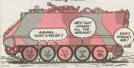
Just because roadwheel arms 4 and 5 have plugs instead of lube fittings doesn't mean the arms don't need grease.
