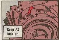
When you set the TU down, protect the AZ lock from damage. Easiest way is to position it with the lock facing up.
