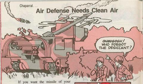
M48A2 Chaparral system to fly true, remember to change the desiccant cartridge in your APU (air purification unit) on schedule.
