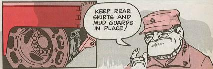
Clean out the mud build-up around the skirts and final drives at halts. Follow the good word on driving in mud. Eyeball Pages 2-370 thru 2-372 of TM 9-2350-255-10-2.
