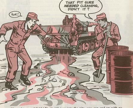
If you let your M110A2's "pit" turn into the pits, you can end up with no commo. Water, dirt, debris and oil can collect and turn the pit into a grungy mess. Besides making for a bad place to work, the mess can knock commo cables out of commission.
