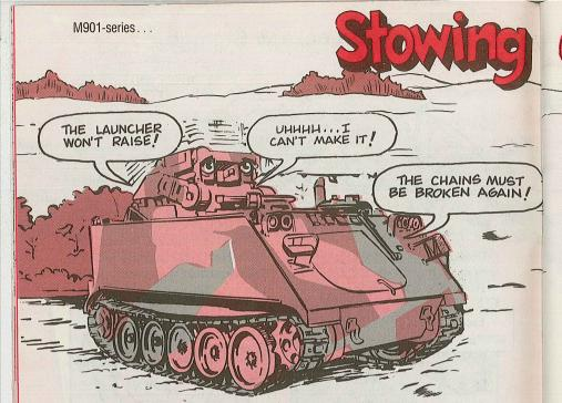
You can break the chains of your M901-series ITV's erector system if you move the ITV when the launcher's not on its supports.
