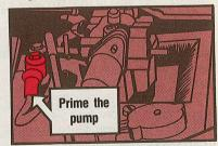
On the other hand, if you find gasoline in your engine's crankcase and you haven't primed it through the carb, have your org mech eyeball the fuel pump's rubber diaphragm. When it dries out and cracks, it lets fuel into the crankcase, too.
