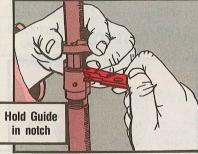
Hold the scraper in position while you turn the collar back beyond the NORMAL position.
