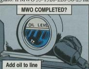
already been completed on your bird, add oil to the indicator line only. If the MWO has not been applied to your bird, add oil until it's 1/8 inch above the indicator line.
