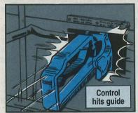
The stress and strain of the sudden stop is centered where the hoses fit on the control.
