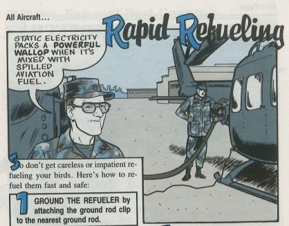
BOND THE REFUELING NOZ-ZLE to the bird before you take the dust cap off the nozzle and the cap off the fill port. It equalizes the electrical charges of the nozzle and the aircraft. If the bird has a receiver for the bond plug, use it. If not, clip it to a bare metal part of the bird.
