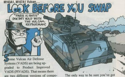
If you use the PIVADS distribution box on a Vulcan, you not only burn out the distribution box but other components as well. The wrong radar unit keeps the radar unit from tracking.
