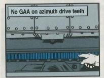
sand, which chews up the teeth. Use the same lubricant for the cranes on the Guided Missile Transporter and the Large Repair Parts Transporter.
