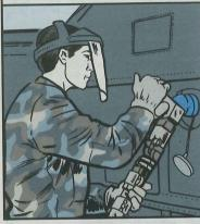
PUT THE NOZZLE all the way into the fill port and lock it into place.
