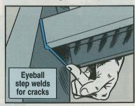
welds for cracking. DS can reinforce the steps with a cross-bar fix. That will hold you until your new ladder, NSN 2540-00-854-4445, arrives.
