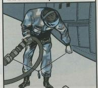
GROUND THE AIRCRAFT by attaching one end of a ground cable to the ground rod and the other end to a bare metal part of the bird. Use the axle of the landing gear or some other unpainted metal part.
