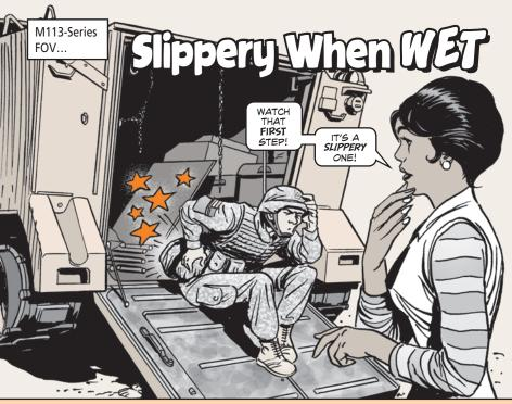
The ramp on your M113-series vehicle is made to load and off-load troops quickly and safely. But safety goes out the window if the ramp's nonslip coating is in bad shape.
