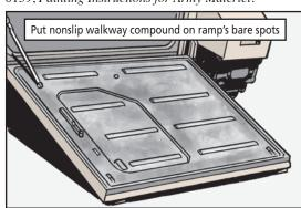
**5.** After the nonslip compound has dried, apply a topcoat of WD CARC paint. Application instructions start on Page 9 of TB 43-0242. Choose the type and color WD CARC paint from the list in App B.
