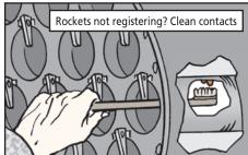
Mark bad tubes. If troubleshooting does turn up a bad tube, mark out its number immediately on the top of the launcher at each end. That way you will remember which tube is bad and will know not to bother loading a rocket in it again.
