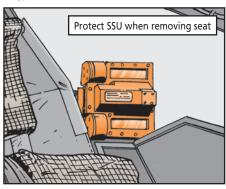
If the mounts are broken, it's over for your bird. It will be red X'd and won't be flying until the SSU mount gets repaired by a depot maintenance contact team.
