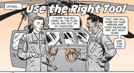
Lechanics, using a hammer and an extension to turn off the main module transmission oil flow is not the way to go.
