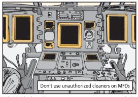
**Do**, at all times, use the authorized glass cleaner, NSN 7930-01-442-5969, and the wipes that come with it. Make a note until the cleaner is added in the next IETM change. This will include procedures for cleaning the MFDs.
