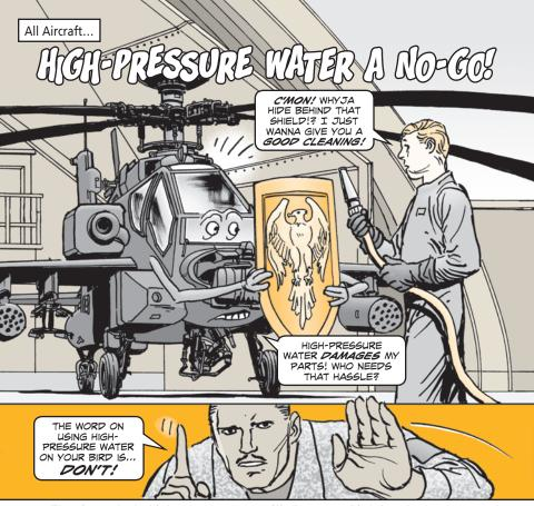
There's no doubt high-pressure water will clean your bird, but the consequences will be costly repairs. High-pressure water damages wire bundles, seals, the finish, connectors, electrical components, and washes grease out of lubricated parts.
