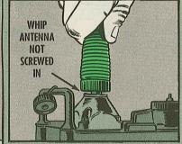
You might even put a sliver of rubberband or pencil eraser on the threads before screwing it into its receptacle.
