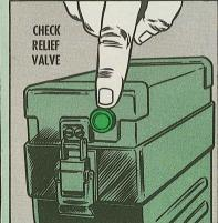
relief valve in the CY-2562, to keep hydrogen gas from getting into the radio chassis and exploding.
