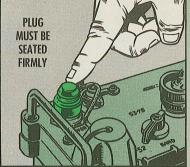
is being taken out of its vehicle, seat the plug or cap firmly.
