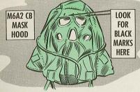
The hood's eyering opening has a black mark at the top. That mark has gotta line up exactly with the "dimple" in the mask eyering.
