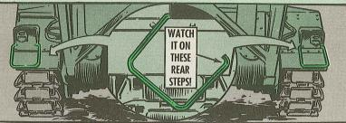
LEAKING SPADE CYLINDERS—Using the polished spade cylinder rod as a step gets the rod dirty and scratched. This damages the O-ring seal and causes leaks at the spade cylinder. For now, keep your feet off the cylinder and protect the polished cylinder rod with an oily rag when possible.
