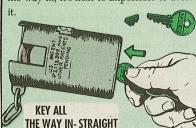
2. Twist the key 45 degrees clockwise. E-a-s-y does it. Never use the key ring or pliers for added leverage.
