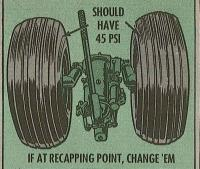
You should have 45 PSI air pressure in the tires. If the tires are cut or worn to the recapping point, change 'em.
