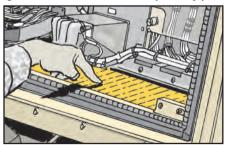
If dirt builds up inside the Sentinel, electrical connectivity suffers, plus components can overheat. Use tech wipes and **isopropyl** alcohol to clean out the inside of the compartment. Don't use plain rubbing alcohol because it takes off the protective finish. Don't use water, either. It will cause corrosion and connectivity problems. Clean the cable connections with isopropyl alcohol, too.
