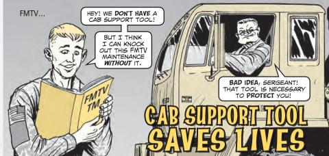
Experience is never a substitute for the education you get from your vehicle's TM. Sadly, a seasoned mechanic found that out the hard way. While replacing the cab hydraulic cylinder on an M1078 LMTV, the 3,000-lb cab dropped on him. He didn't survive.
