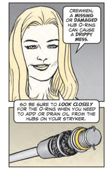
A missing or damaged O-ring means you won't get a good seal and the hub can leak. If the leak's bad enough, the hub goes dry and the bearings can burn up.
