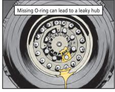
Replace missing or damaged O-rings with NSN 5330-12-156-4524. If the old O-ring is undamaged, wipe it off before reinstalling the plug. If there's a lot of dirt or sand on the O-ring, it won't seal properly and you've got leak problems all over again.
